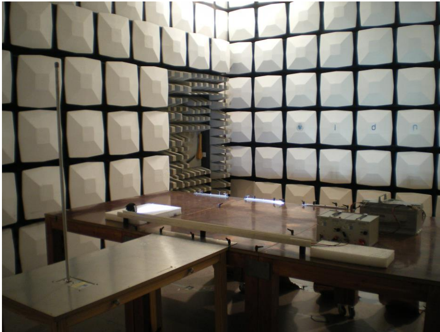
Figure 18. RE Test – CISPR 25. Test Setup applied for 12V from 100 kHz to 30MHz.
