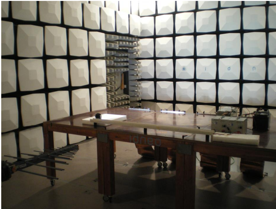
Figure 24. RE Test – CISPR 25. Test Setup applied for 24V from 200MHz to 1GHz.
