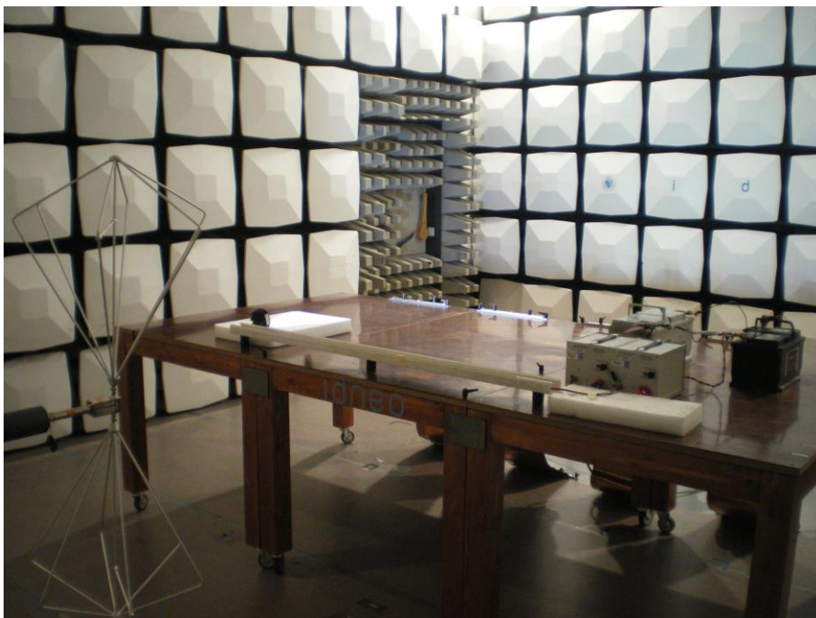
Figure 23. RE Test – CISPR 25. Test Setup applied for 24V 30MHz to 200MHz.
