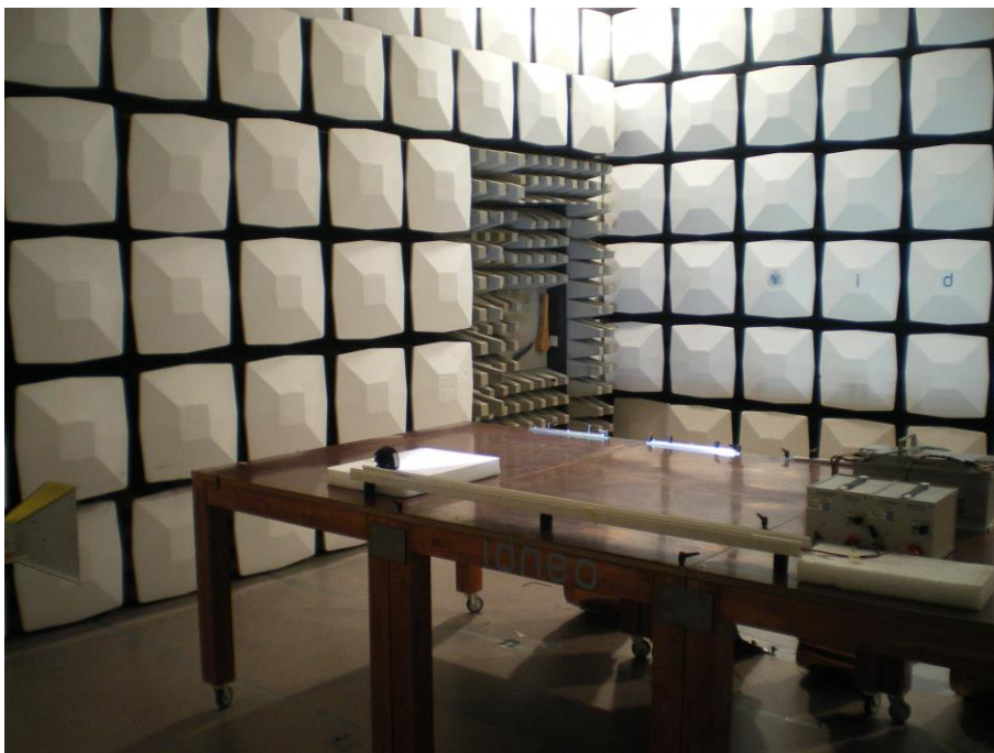
Figure 21. RE Test – CISPR 25. Test Setup applied for 12V from 1GHz to 2GHz.
