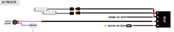
Customer's have the option to connect to a positive battery or ignition feed. Connecting to the ignition feed, the light will only operate with the ignition turned on.
