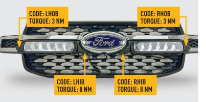
**INSTALLATION PROCESS** - Install should be completed with the grille left on the vehicle.
