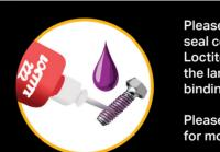
Please use a thread seal compound (i.e. Loctite 222) to protect the lamp fastener from binding over time.
