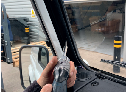
3. Carefully remove rear view mirror and base.
