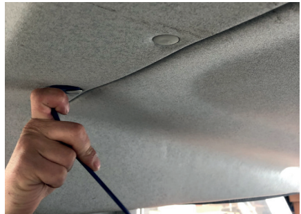
6. Remove the push-in clips from around the headlining.
