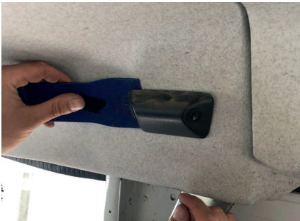
5. Remove ultra sonic module.
