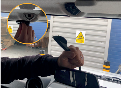
5. Remove ultra sonic module.
