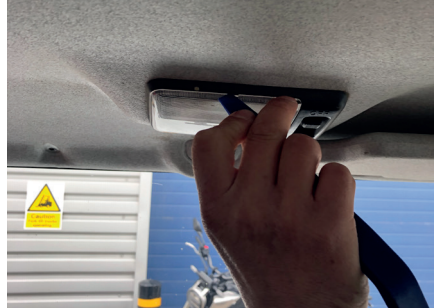
6. Remove the push-in clips from around the headlining.
