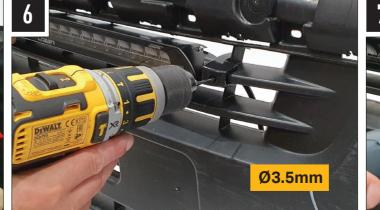
Please use a thread seal compound (i.e. Loctite 222) to protect the lamp fastener from binding over time.
