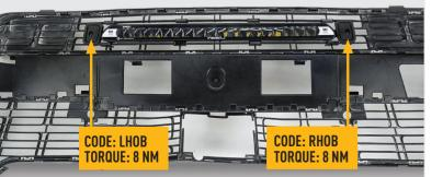
**INSTALLATION PROCESS** - Linear-18 shown for illustration purposes. Install should be completed with the grille left on the vehicle.
