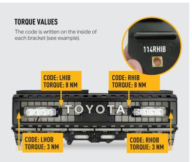
INSTALLATION PROCESS - Install should be completed with the grille left on the vehicle.
