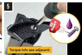
Please use a thread seal compound (i.e. Loctite 222) to protect the lamp fastener from binding over time.
